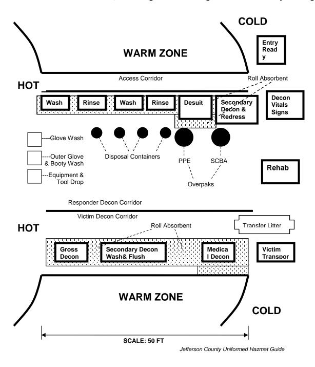
The Decon Officer will orient arriving Hazmat team members by placing two traffic cones to indicate the entry width of the three decontamination corridors.
